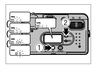
Press the DATE button to select the next number blinking in the order Year  $\rightarrow$  Month  $\rightarrow$  Day  $\rightarrow$  Hour  $\rightarrow$  Minute. Press the  $\circlearrowleft$  button 1 to correct the numerals blinking in the liquid crystal display. If you press the DATE button 2 at this time, the blinking numerals to be corrected will change in sequence from Year  $\rightarrow$  Day  $\rightarrow$  Hours  $\rightarrow$  Minutes.
